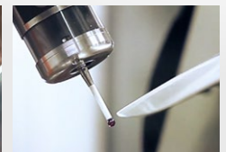
The probing tool checks & corrects the toolpaths exactly
