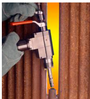
Only 1.5" wide for single boiler tube beveling
