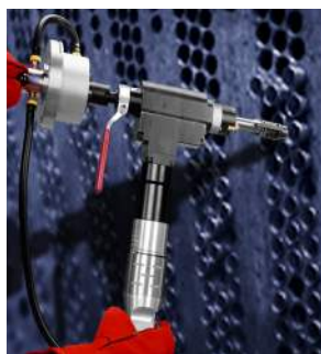
The air clamp increases production and minimizes operator fatigue
