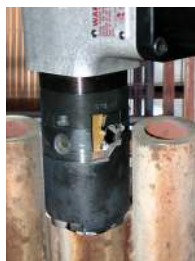
The ESCO patented membrane and overlay removal heads use round tapered inserts that can be rotated when worn and install and removed with a tap from a hammer.
