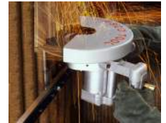
The boiler tube panel saw works on the same track as the straight-thru models.
