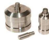
Pilots center the tool and keep it square to the tube. A properly sized pilot is .015" to .030" under the tube I.D. This tolerance ensures smooth operation, long blade life and chatter free bevels.
