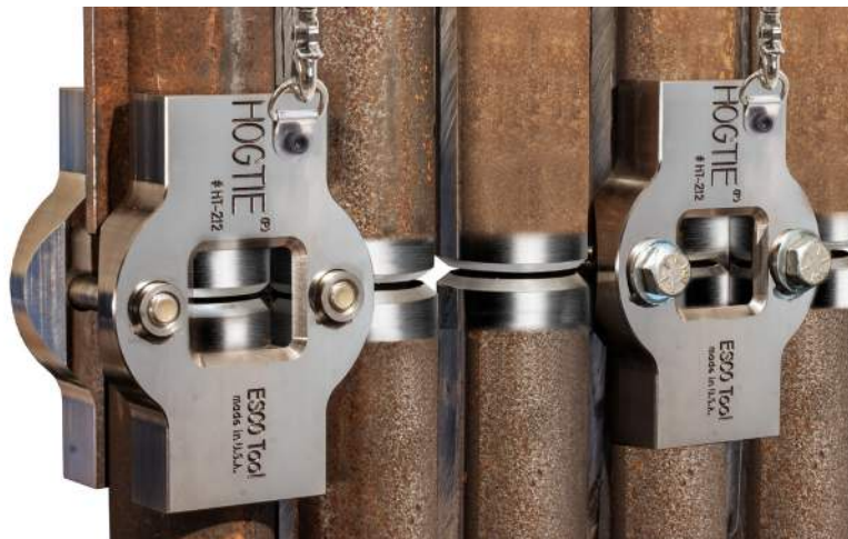
HOG TIE® tube alignment tools speed waterwall boiler tube fit-up and helps reduce tube joint failure due to misalignment.
