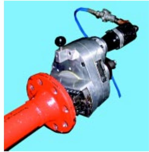
Mactech's 12-24 SP and 24-36 SP End Prep Lathes can form bevel, face and counterbore pipe. They produce precision end preps on tube and pipe ranging from 12" to 24" and 24" to 36" I.D. (respectively) and single-point bevel pipe and face flanges out to 24" and 36" O.D.
